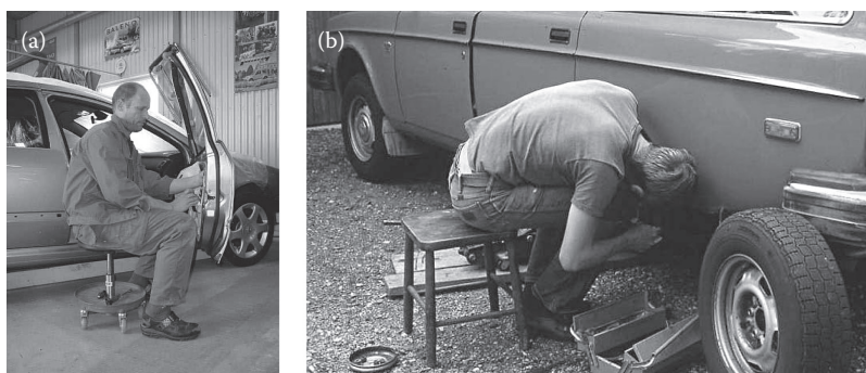
FIGURE 4.9 A simple moveable step (a) allows work to be carried out without needing to twist or stoop in order to gain access. On the other hand, working on a step—depending on the work height—may also mean that it is more difficult to gain access (b). Photo (a): Christer Spångberg; (b): Karin Harms-Ringdahl.
